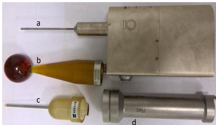
**Figure 1.** The XRS and applicators of 3 different shapes. (a) the XRS, (b) the spherical applicator, (c) the Needle applicator, (d) the flat applicator.
